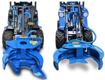
Two models are available: with fixed blade for trunks up to 10 cm diameter and with hydraulic blade for trunks up to 15 cm diameter. Through the reach of the MultiOne's boom, this unit can also be used to prune branches, and clear scrub growth in places difficults to reach.
