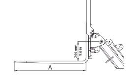
allow the width of the forks to be easily adjusted by as much as 1 m / 39 in (70 cm / 27.6 in on C895120). Optional bolt on back stop provides additional safety. MultiOne is an excellent machine for load handling thanks to the precise steering and drive control. Compared with a conventional forklift truck MultiOne is superior when working outdoors and on uneven terrains, on all seasons.
